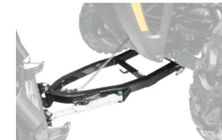
PLOW PUSH FRAME AND FRAME MOUNT (2436-390)
